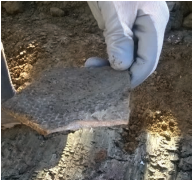
Figure 7. Asbestos-cement sheet and bonded ACM in soil.
