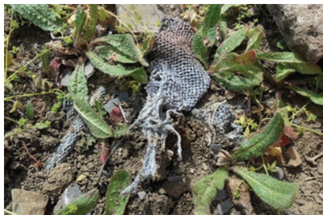
■ Figure 8. Decorative coatings containing asbestos in soil.
